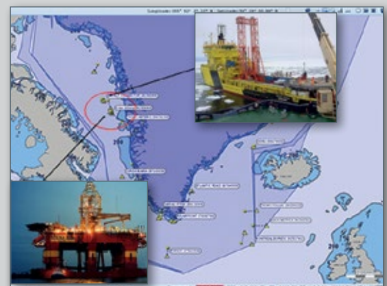
Figure 11: Screenshot of the EU LRIT CDC including the custom coastal standing order which is activated in the DDP and showing vessels in the area of the offshore installation
