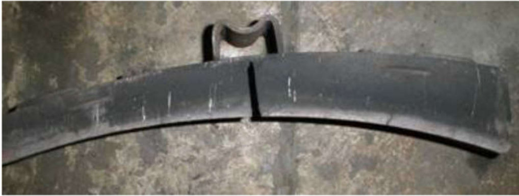
Figure 1: Organic brake blocks: 'White layer' in the rubbing surface near to the surface area, up to 10mm thick, friction carbon deposits [UIC Leaflet e541-4, 3. Edition]
