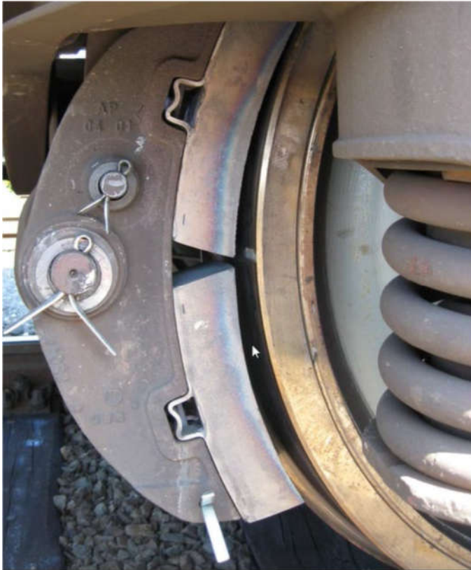
Figure 3: Sintered brake blocks: White-blue layer' in the rubbing surface, up to 10mm thick [UIC Leaflet e541-4, 3. Edition]
