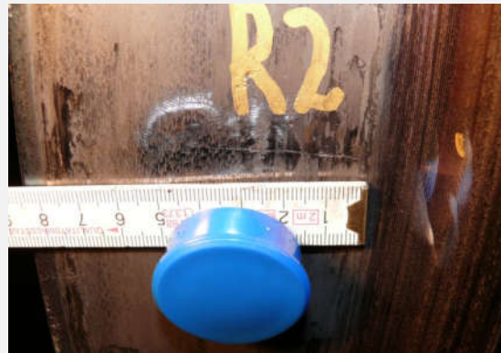
Example for single cracks on the wheel tread by visual inspection
