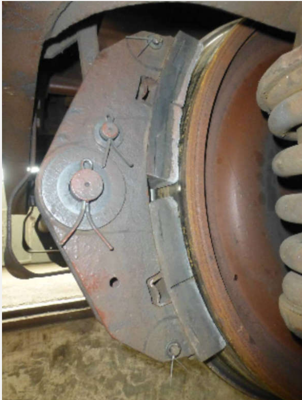
Cast iron brake blocks - Melted brake block
